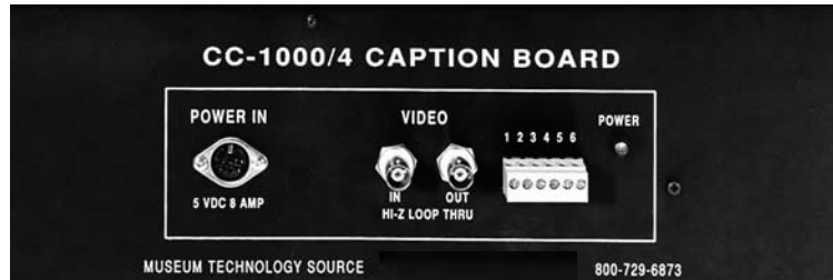
Detail of Rear Panel of the CC-1000 Captioning Board showing connections
